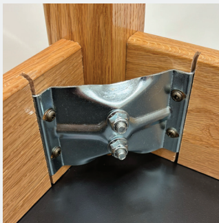
Heavy duty double bolted steel corner braces with self-locking nuts.
